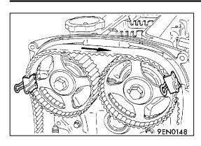
(6) Secure the timing belt with a paper clip at the illustrated position.
