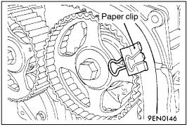
(4) Fit the timing belt to the intake camshaft sprocket and secure with a paper clip at the illustrated position.
