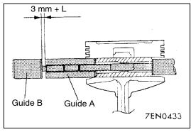
(7) Screw the guide B into the guide A until the gap between both guides amounts to the value L obtained in step (2) plus 3 mm.
