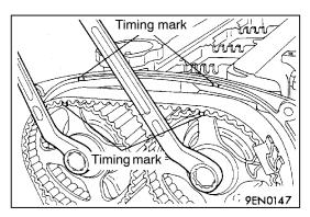
(5) Use two wrenches to fit the timing belt to the exhaust sprocket while aligning the timing marks.
