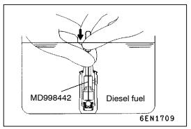
(3) While gently pushing down the internal steel ball using special tool, move the plunger through five to ten strokes until it slides smoothly. In addition to eliminating stiffness in the plunger, this operation will remove dirty oil.
