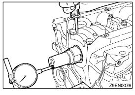
(8) After installing the bearing caps, make sure that the crankshaft turns smoothly and the end play is correct. If the end play exceeds the limit, replace crankshaft bearings.
