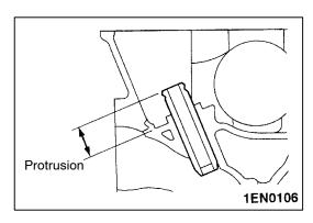
(3) Press-fit the valve guide until it protrude specified value (SOHC: 14 mm, DOHC: 19 mm) as shown in the illustration.
