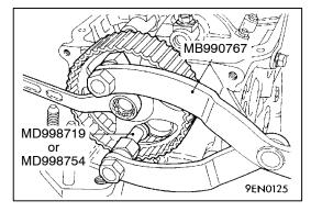
**◆B** CAMSHAFT SPROCKET BOLT REMOVAL
