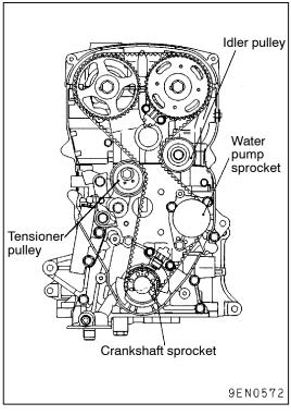
(7) Fit the belt to the idler pulley water pump sprocket, crankshaft sprocket and tensioner pulley in that order.
