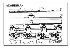
(8) Tighten the fasteners of the delivery pipe and injector assembly to the specified torque in the order given in the illustration.
