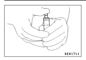
(15) Remove the lash adjuster from the container, then stand the lash adjuster with its plunger at the top. Push the plunger firmly and check that it does not move. Also, check the lash adjuster's height matches that of a new lash adjuster.
