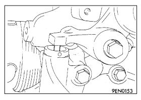
(17) If the wrench cannot be pulled out lightly, repeat the steps (12) through (15) to obtain appropriate belt tension.
