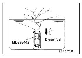
(8) Stand the lash adjuster with its plunger at the top, then push the plunger downward firmly until it moves through its greatest possible stroke. Return the plunger slowly, then release the steel ball and allow the pressure chamber to fill with diesel fuel.
