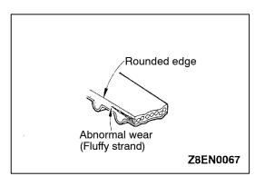
(6) Abnormal wear of belt sides. The sides are normal if they are sharp as if cut by a knife.
