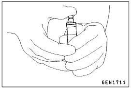
(9) Remove the lash adjuster from the container, then stand the lash adjuster with its plunger at the top. Push the plunger firmly and check that it does not move. Also, check that the lash adjuster's height matches that of a new lash adjuster.
