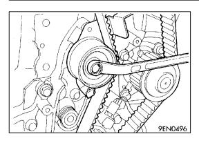
(6) Slightly loosen the tensioner pulley fixing bolt which is tightened temporarily to tighten the belt by a force of the tensioner spring.
