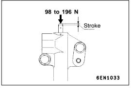
(4) Press the rod by a force of 98 to 196 N and measure the rod stroke. If not within the standard value, replace the tensioner.
